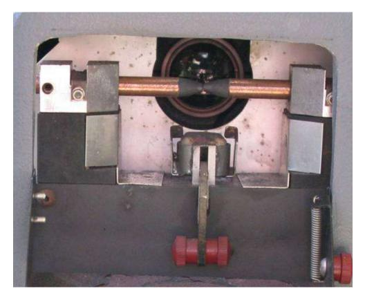
The electrodes are then adjusted to where they barely touch which when power is on an electric arc will be generated. The specs on the shield wall are due to flying hot/molten particles.
