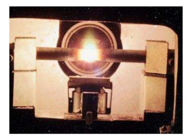
The arc is initiated and the sample laden boat is slowly raised into the arc.
