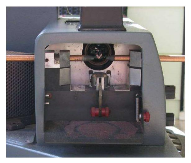
The copper coated carbon electrodes must be adjusted to a predetermined – centered - position prior to creating the arc. The red knobbed positional bracket is in the down (out of the way) position.
