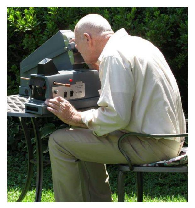
While the mineral sample is being melted and/or vaporized I am looking into the lens viewer to see what elements may be present. Since these images were taken I have purchased a long/large weather resistant outdoor table that allows me to have all the associated expendables, hand tools and note papers.
