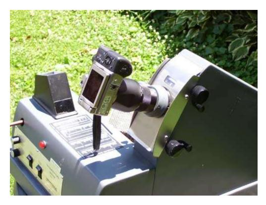
The Vreeland equipped with a Cannon 12mp digital camera to record either single images or video clips of the generated spectrum lines as the mineral sample is melted and/or volatilized. With the camera I have what I consider to be a decent spectrograph and the saved images allow me to review the results.
