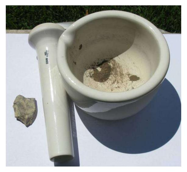
Before a test can be accomplished I use a ceramic mortar/pestle to pulverize the rock (at left).
