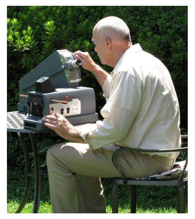
I am adjusting the film to a specific element number. The numbers can be seen in the small window just above the viewing lens. Due to the need of adequate lighting for these pictures and not be exposed to the fumes I conduct these assays outside.
