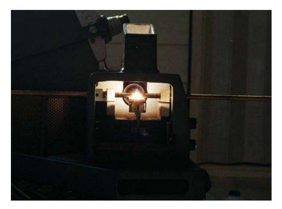
The sample is totally submerged in a bath of the hot (2000+F to 5000+F) electric arc. Fumes exit out the chimney. Normally, the electric arc cannot be seen because a flip door is closed.
