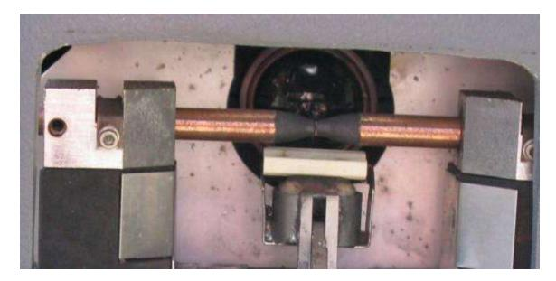
The boat is raised to about this position after the electric arc is generated.
