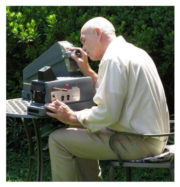
I am watching as I adjust the sample into the electric arc. There is a welder's type lens mounted on the vent hood that allows me to see the sample moving into the electric arc without damaging my eyes.
