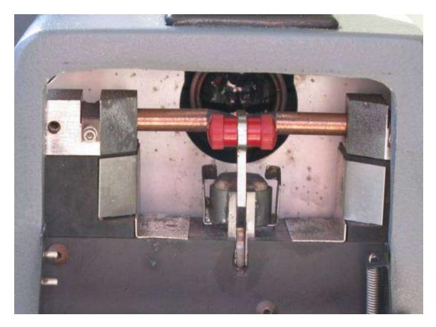
This image shows the red knobbed bracket in up position creating the exact centered position necessary for the arc light to sent through the lens behind the electrodes. The lens transmits the focused light to a slit then to the diffraction grating then to the viewer lens.
